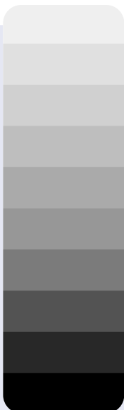
When halftones are shot, a density guide, or gray scale, that displays the entire range of density values is laid beside the photo being shot. A comparison is made between the original and the resulting halftone to ensure there is no loss of tonal values.
